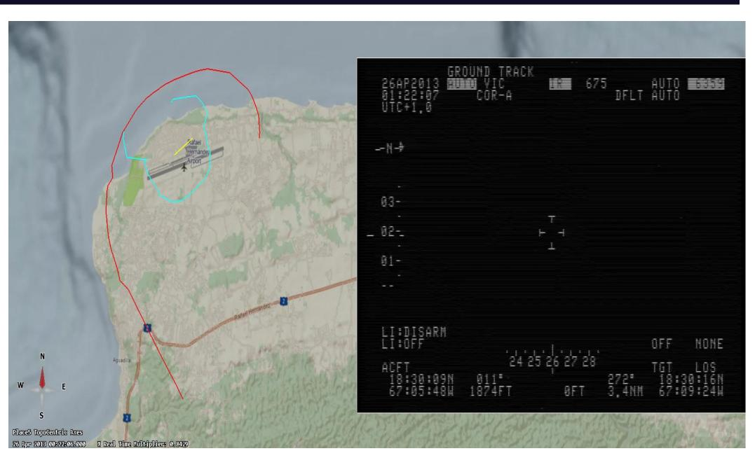
Vector analysis is used to plot the line of sight of the sensor as a function of time. Using a closest-approach method, a track of the object can be estimated
